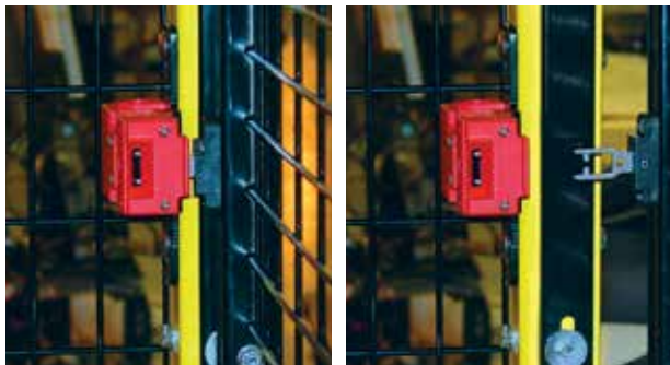
Safety interlock engaged
